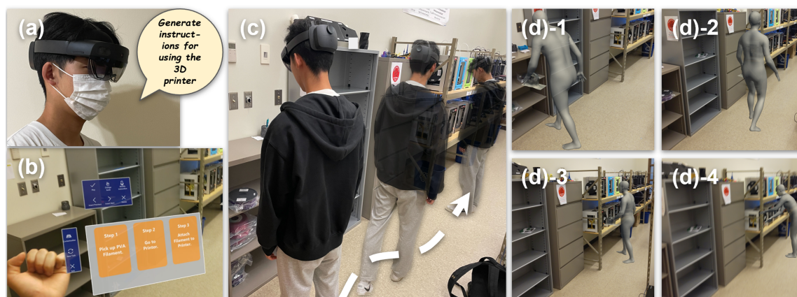
Figure 1: An overview of CARING-AI system authoring workflow. CARING-AI enables authors to create contextualized AR instructions through generative AI. (a) Using CARING-AI, authors first speak their intended instruction content, (b) then the corresponding step-by-step instructions are generated in text. Authors interact with the interface to modify the textual instructions and group them. (c) Then the authors provide contextual information to the instructions by walking in the environment and taking screenshots with the AR HMD. (d) Finally, CARING-AI generates step-by-step humanoid avatar demonstrations of the AR instruction situated in the context.
